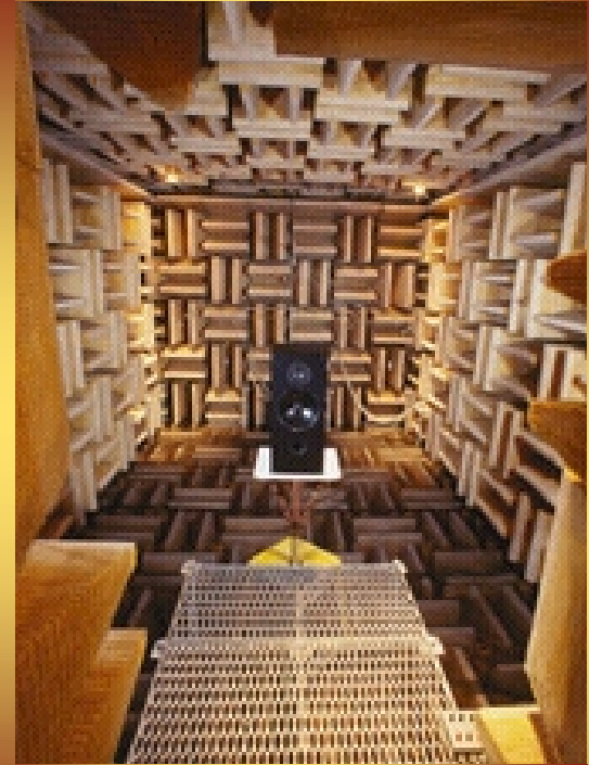
Anechoic Chamber at IMS – A primary facility in the growth of Canada's loudspeaker manufacturing industry.
