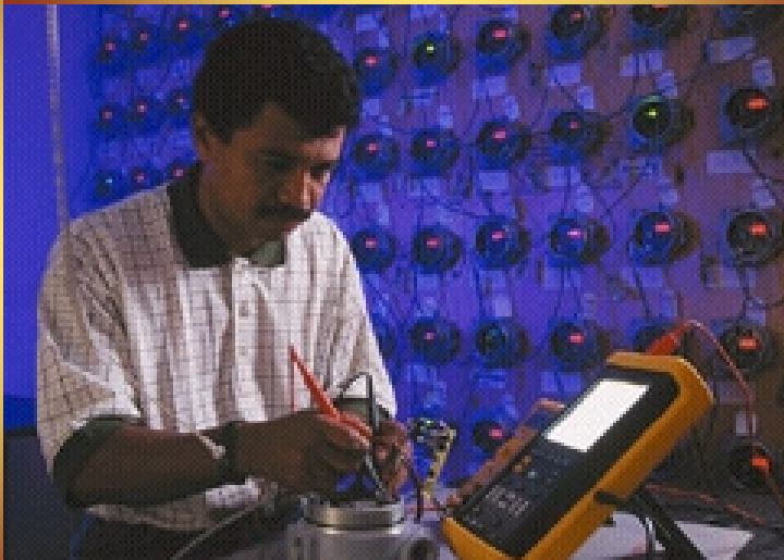
ICPET - Thin film chemical sensors monitor minute levels of gas and vapour.
